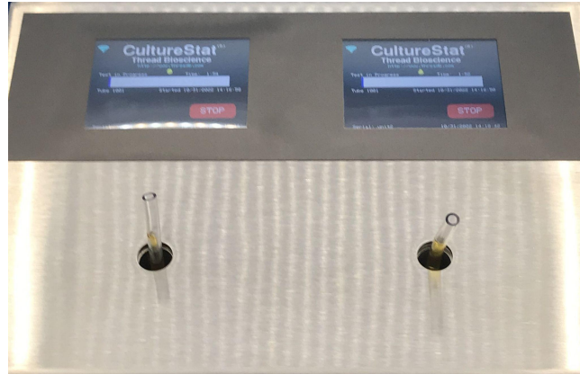
(Example of how ampoules should be placed in device)
